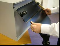
Line up the castor base. Please note that the lip on the castor base fits underneath the lip on the front of the cabinet as shown.
