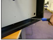
Using a cross head screwdriver remove the 2 screws holding the plinth in place.
