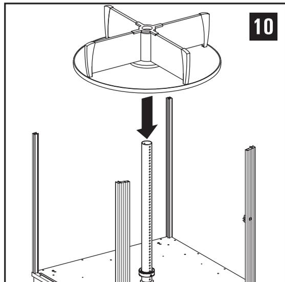
The plastic parts must click into place in 4 positions respectively, giving an audible sound.
