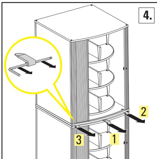
We recommend having 4 people assist in placing the **LockFile®** elements on top of each other. Using 3 distance wedges, place the upper element on top of the lower one and move it into the proper position. The locating pins fit exactly in the hexagonal holes of the Allen screws. Position the **LockFile®** elements in such a way that they are exactly flush on top of each other.
