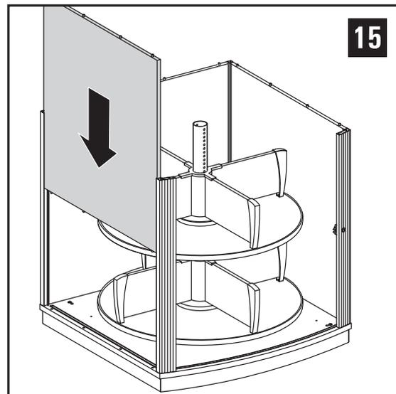
Adjust the level distance as required. Max load per level: 90kg
