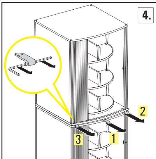
We recommend having 4 people assist in placing the **LockFile**<sup>®</sup> elements on top of each other. Using 3 distance wedges, place the upper element on top of the lower one and move it into the proper position. The locating pins fit exactly in the hexagonal holes of the Allen screws. Position the **LockFile**<sup>®</sup> elements in such a way that they are exactly flush on top of each other.
